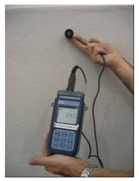
Figure 26 – Measurement in the tunnel, using the photo-radiometer
