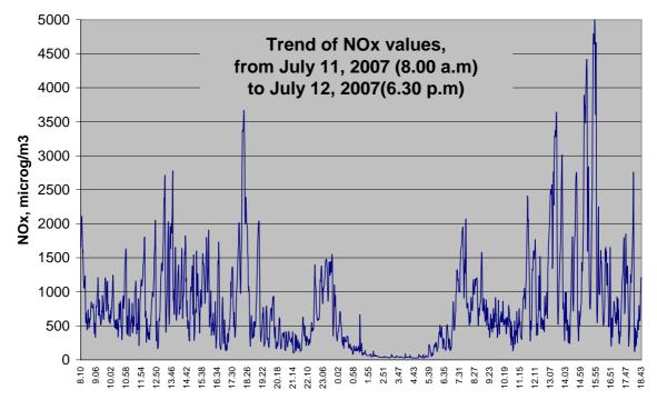
Figure 36 – Trend of NOx values, in the centre of the tunnel, including a nocturnal data collection
