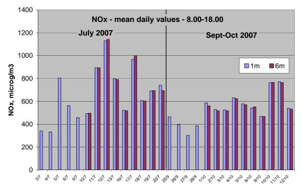
Figure 38 - Comparison of  $NO_x$  values, in the centre of the tunnel (1 m and 6 m)
