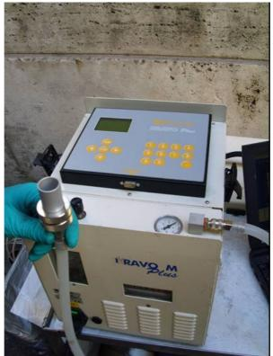
Figure 48 – TCR Tecora pollution check equipment, over the NOx analyser
