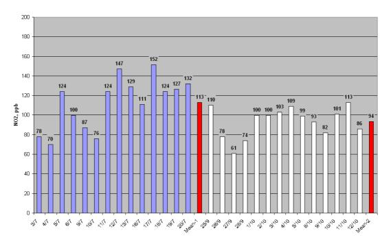
Figure  $41 - NO_2$  values in the centre of the tunnel, 1 m
