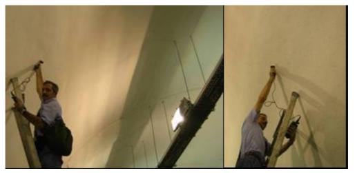
Figure 25 – Measurement of the light intensity, in the tunnel
