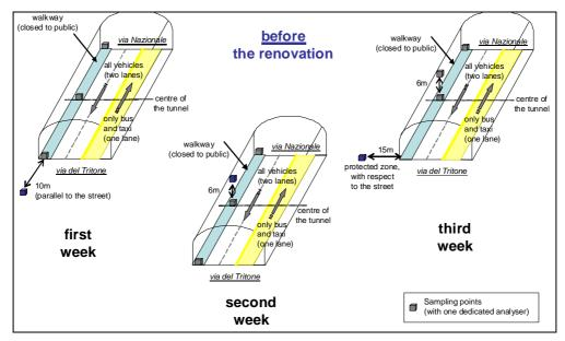
Figure 17 – Positions of NO<sub>x</sub> analysers, during the first campaign
